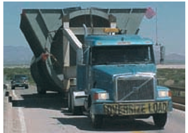
Oversized one-piece stack in transit to Arizona
